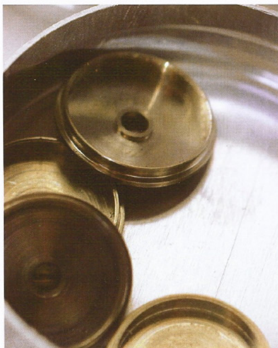
from top—A collection of Arabic numerals destined for Vyskocil watch dials; tooling of a wheel; barrels ready for assembly. The maker manufactures nearly all of the parts that go into his watches.
